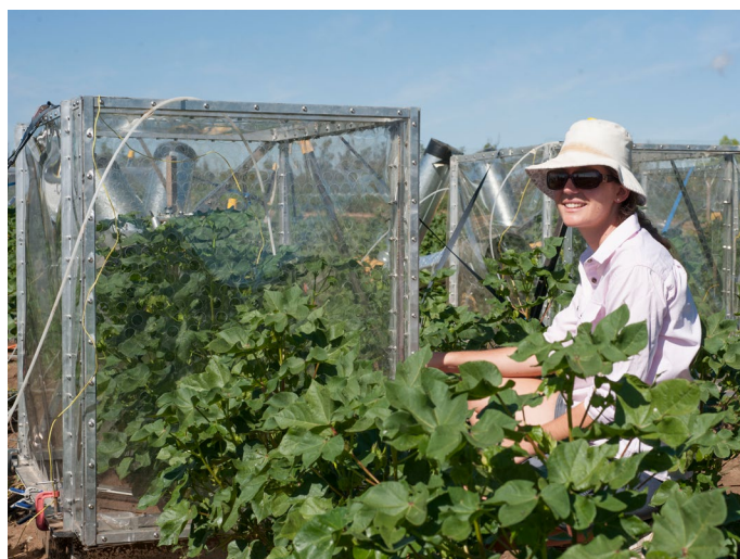
Figure 3: Using Canopy EvapoTranspiration and Assimilation (CETA) chambers in the field at Narrabri, NSW to generate warmer and higher CO 2 environments for field-grown cotton
