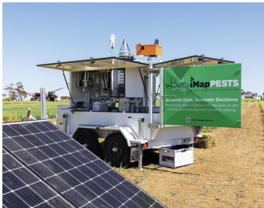
The Sentinel, a mobile surveillance unit offers optimal sampling of airborne fungal spores and insects.
