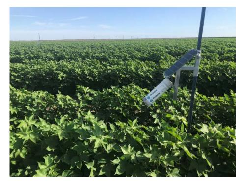
Figure 2: Canopy Sensor in action
