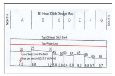
Figure 1: Difference in head height and flow rate across a field.
